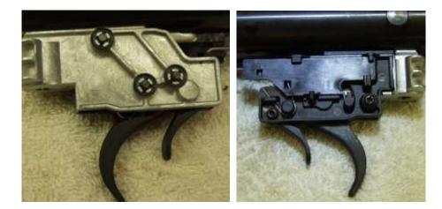
Take notice of the bear trap link (the long wire attached on one end to the cocking linkage and other end connected the plastic guide/slide on the side of the trigger). You will see on the side of the plastic guide/slide and a torsion return spring. Carefully note the orientation of the torsion return spring and how it is installed and to be reinstalled. Remove this spring and set it aside.
