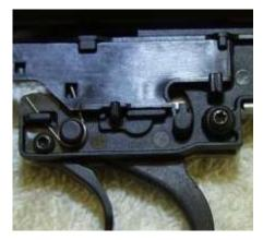
NOTE: You will need either a small Phillips screwdriver or the #8 Torx screw driver or bit to remove the cover screws. That said though, they are screwed into plastic and a person can take a small pocket blade screwdriver and grind it down just a tiny bit at a time to a good fit catch the screw and unscrew them. We did it to test it and it was no problem as they are not real tight due to being screwed into plastic and are so small.
