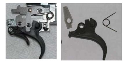
Remove the little metal bear trap block that sets on top of the plastic trigger. Note it's orientation on the trigger.
