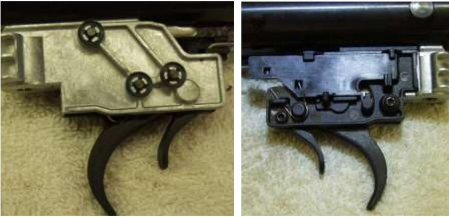
Take notice of the bear trap link (the long wire attached on one end to the cocking linkage and other end connected the plastic guide/slide on the side of the trigger). You will see on the side of the plastic guide/slide and a torsion return spring. Carefully note the orientation of the torsion return spring and how it is installed and to be reinstalled. Remove this spring and set it aside.
