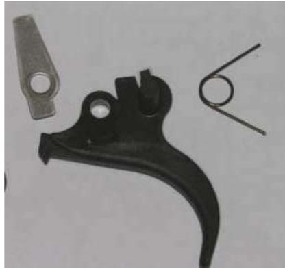
Remove the little metal bear trap block that sets on top of the plastic trigger. Note it's orientation on the trigger.
